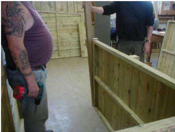
Attach the right hand corner post to the front panel making sure that it is flush to the inner corner of the post.
