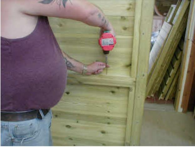
Screw the upper and lower back panels together as shown
