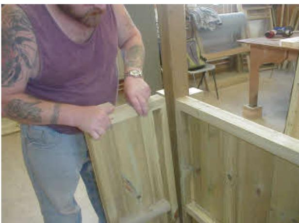
Place the corner return panel on the post and screw into place.
