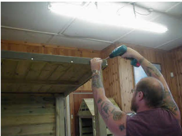
The roof can now be screwed to the front posts through the **front** of the roof.
